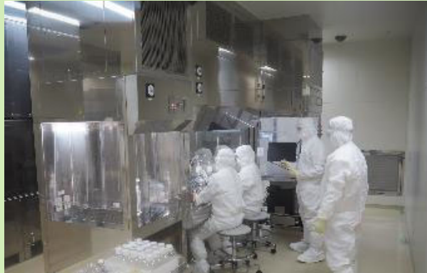
“Aseptic room” + Safety cabinet
